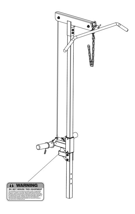
The warning labels shown here have been placed on the Rear Base. If the labels are missing or illegible, please call customer service at 1-800-999-8899 for replacements. Apply the labels in the location shown.
