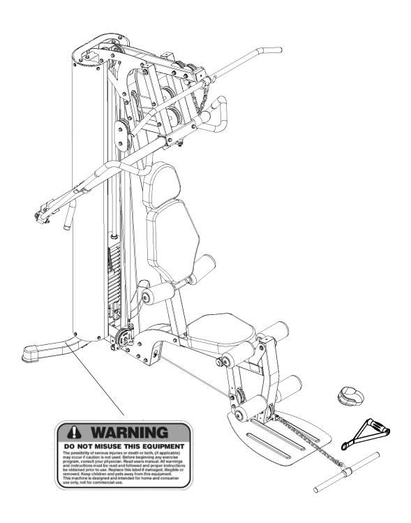
The warning labels shown here have been placed on the Rear Stabilizer and Upper Frame. If the labels are missing or illegible, please call customer service at 1-800-999-8899 for replacements. Apply the labels in the location shown.
